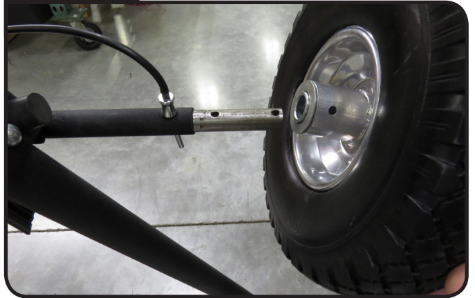
SLIDE WHEEL ONTO AXLE
