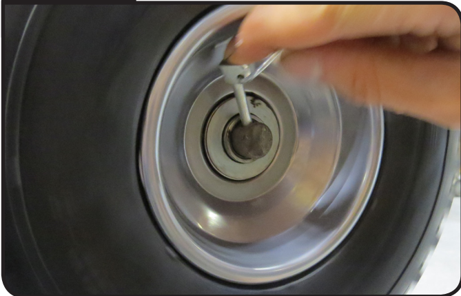
INSERT LOCKING PIN THROUGH HOLE IN AXLE
