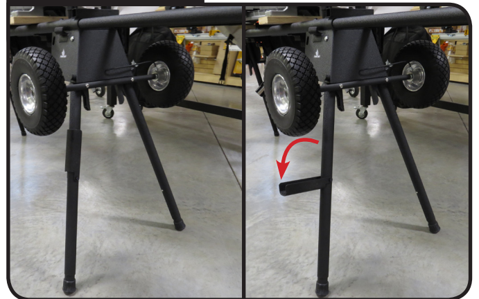
LUMBER RACKS CAN BE FOLDED OPEN TO SUPPORT EXTRA LUMBER
